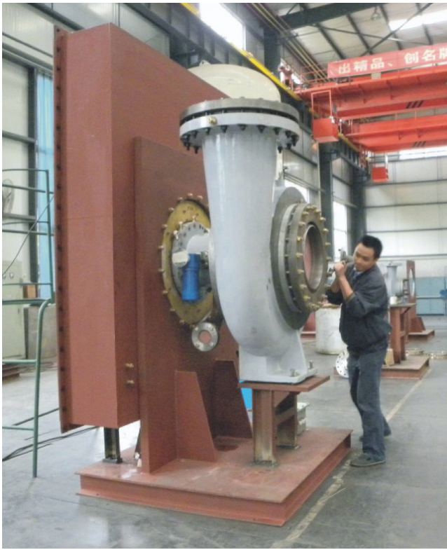
处理量达 93500Nm 3 /h 增压透平膨胀机 (国内最大) Booster Turbo-expander with the capacity of 93,500Nm 3 /h Biggest Capacity in China
