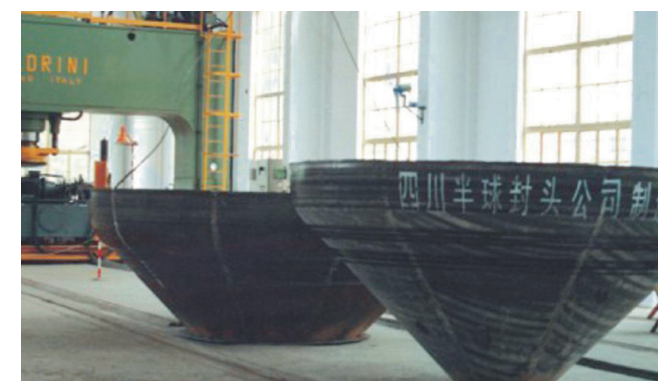
旋压大型锥封头 Large-sized Spun Conical Vessel Head
