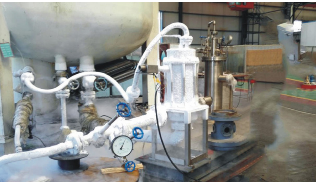
70-120m 3 /h 无机封潜液转注泵 (LNG、LN2、LAR) 70-120m 3 /h Submersible Liquid Transfer Pump (LNG, LN2, LAR) Without Mechanical Seal
